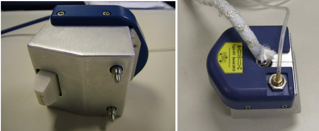
High temperature weld probe with forced air cooling for longer contact times
