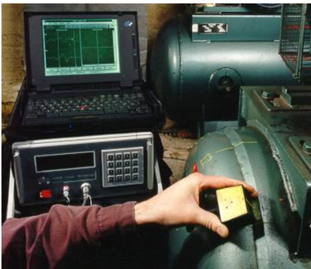
Figure 1. ACFM Inspection of pressure cylinder.
