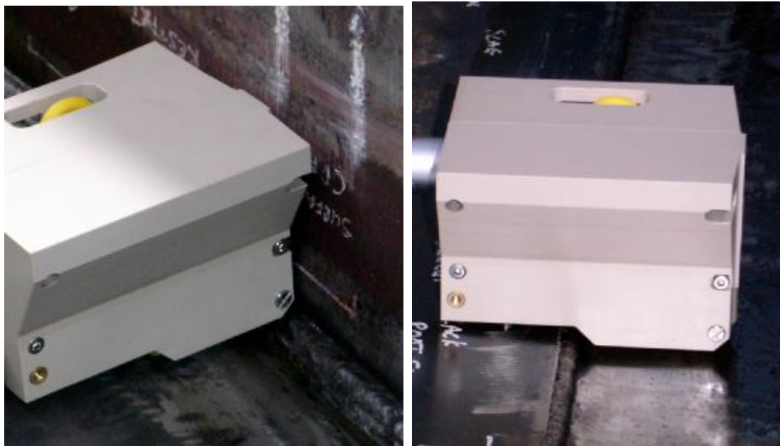
Array probe taken out of trolley to show deployment positions on fillet and lap welds
