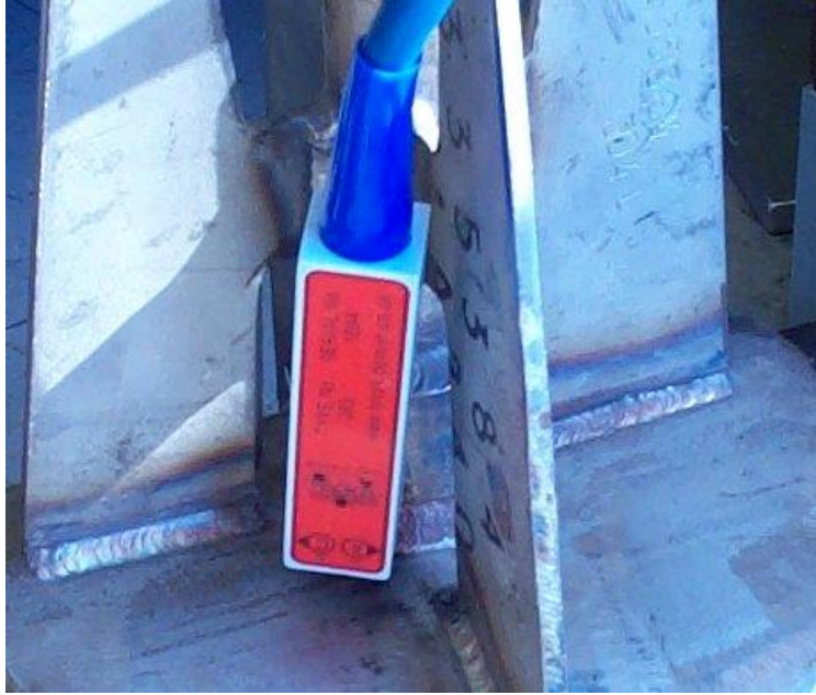
Amigo high frequency probe inspecting Duplex weldolet
