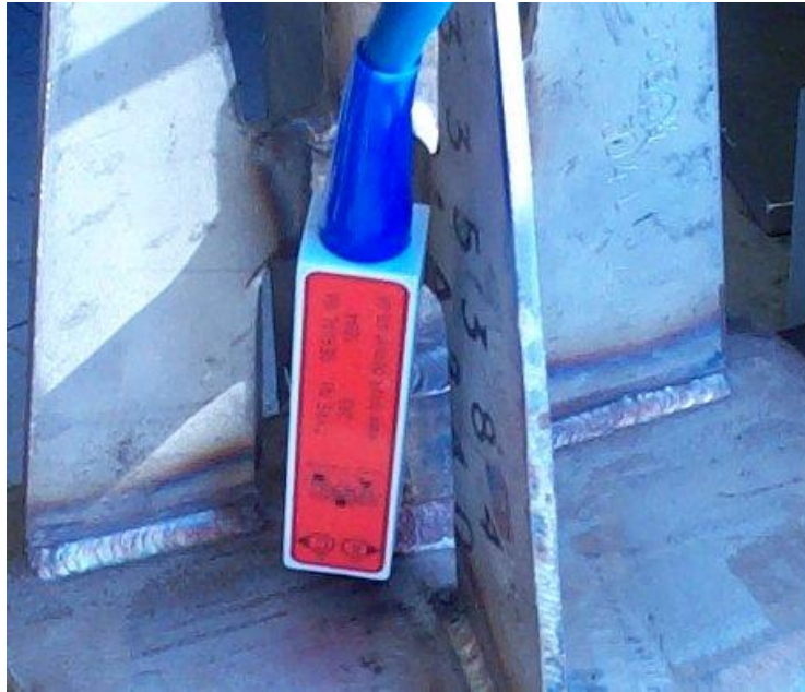
Amigo high frequency probe inspecting Duplex weldolet
